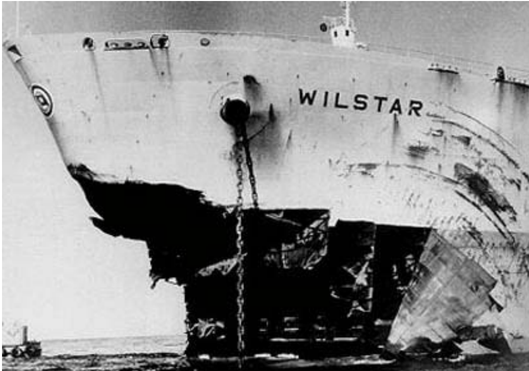
The Norwegian tanker Wilstar was hit by a large wave in 1974, which tore open the bow of the ship.
