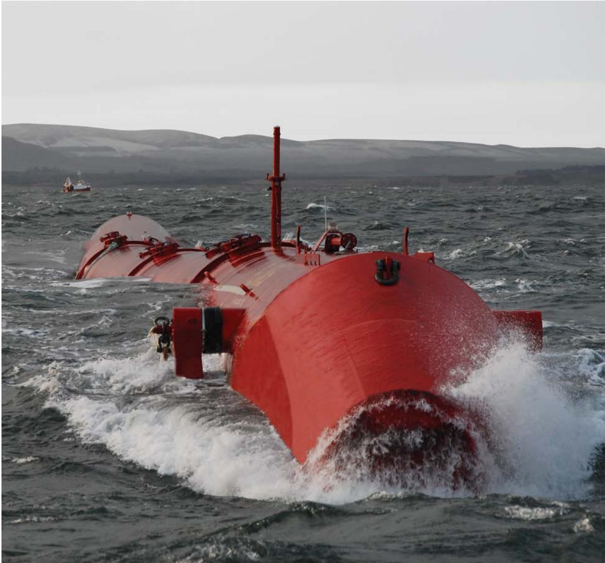
*The Pelamis is the first commercial system using wave power and was installed off the coast of Portugal.*
