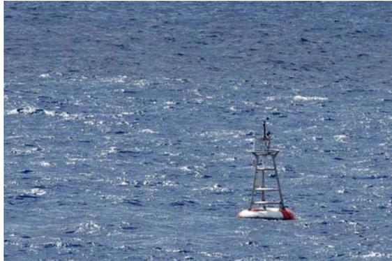
*The international observational buoy, anchored to the bottom in about 12,000 feet of water, at the exact intersection of the Equator (0 degrees) and the Prime Meridian (0 degrees)*
